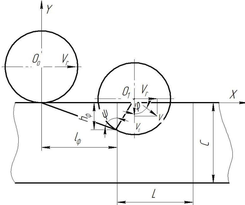
**Figure 5: Scheme of the motion of the particle along the input face of the sowing disk cell**
