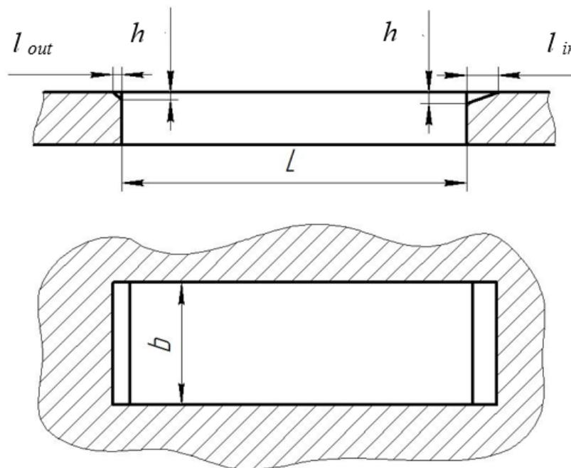
**Figure 8: Scheme of the mesh the sowing disk with input and output chamfers for sowing the seeds of watermelons**
