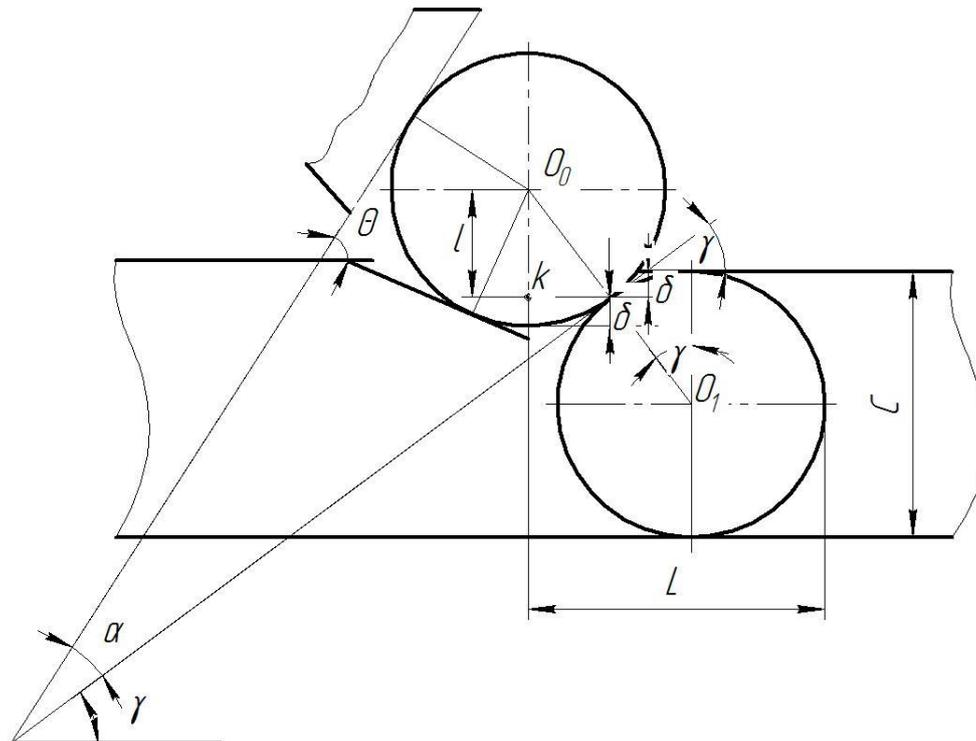
Figure 4: Scheme of pinching a particle by a reflector and another lower particle
