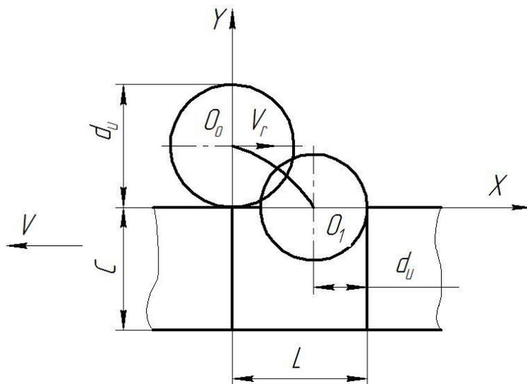
Figure 3: Scheme of motion of a particle on the disk before entering into mesh
