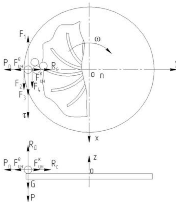
**Figure 6: The scheme of forces acting on the particle, located on the sowing disk and moving in the mass of particles**
