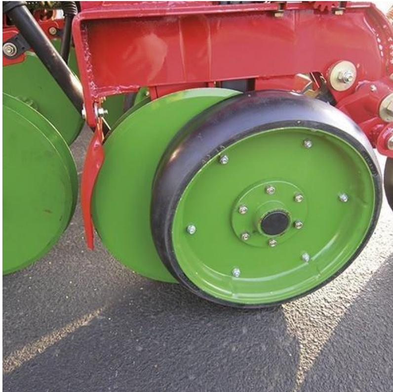
Figure 2: Double disc coulters with replacing a wheel
