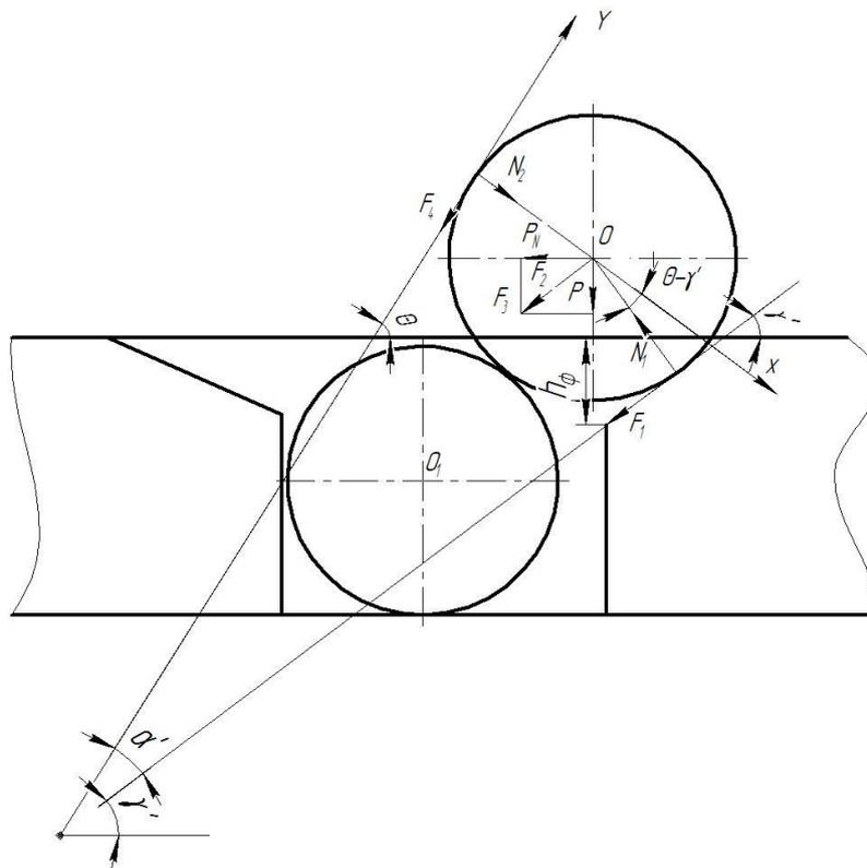
Figure 7: Scheme of the movement of the particle along the output face of the sowing disk
