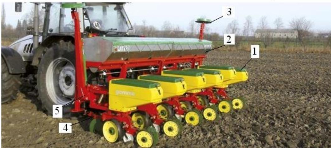
**Figure 1: General view of the GAMMA seeder for the cultivation of tilled crops with a mechanical seeder**
